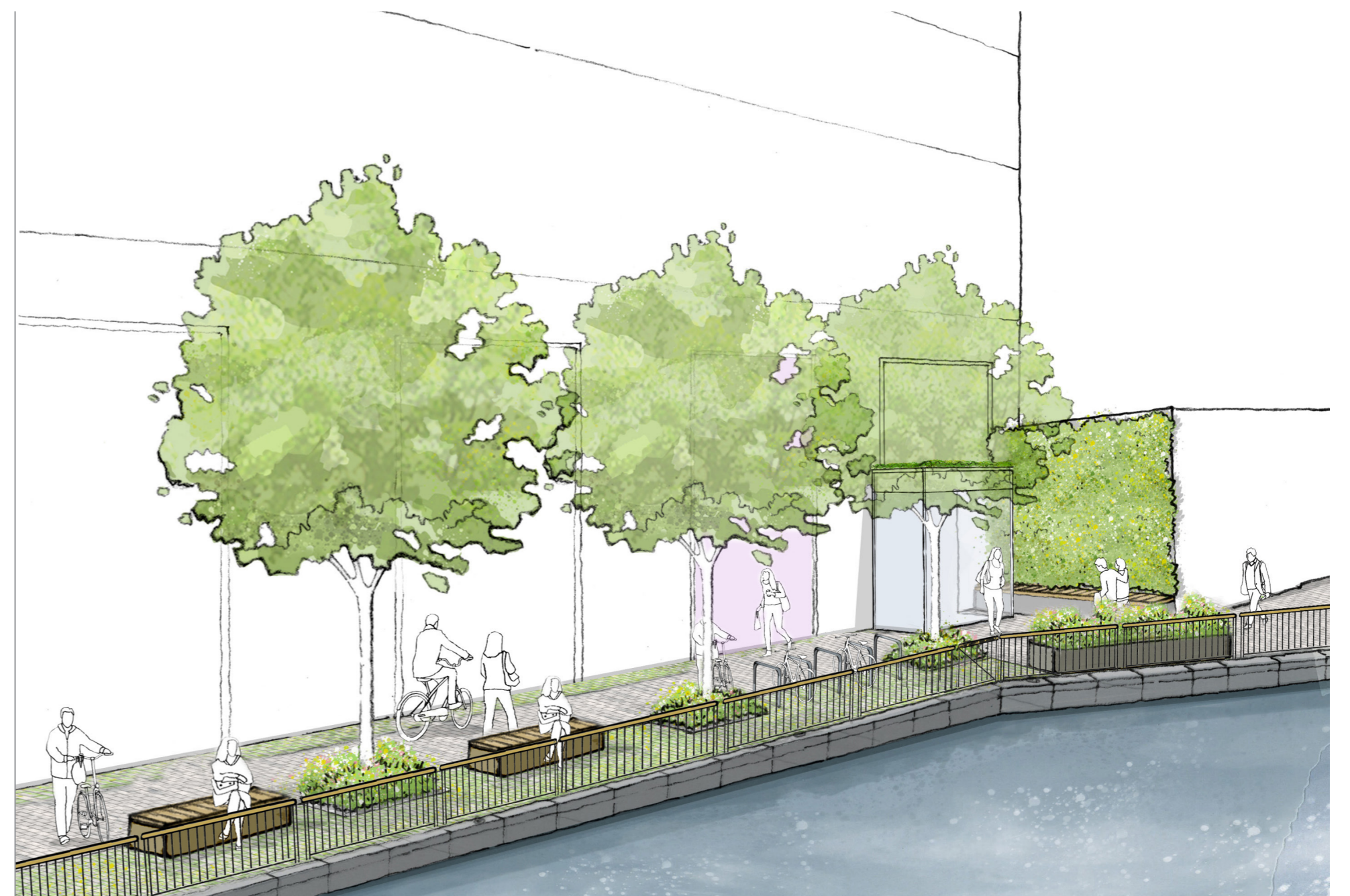
The proposals include tree planting and sustainable drainage features within the canal side path to mitigate risk of pollution running into the canal water
